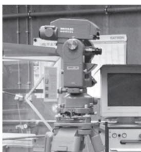
Gambar 7.4 Theodolit Sumber: www.image.google.com
