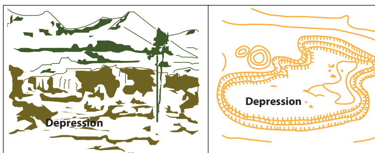
Figure 2.31: A depression and its representation on a contour map
